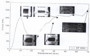
Figure 3: Load Displacement Curve for Specimen 2504.
