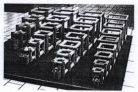
Figure 2: Three-Dimensional Tubular Absorbers before Crushing Tests
