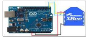
Fig. 3. Iinterconnection of Arduino microcontroller with Xbee module (from Google Images)
