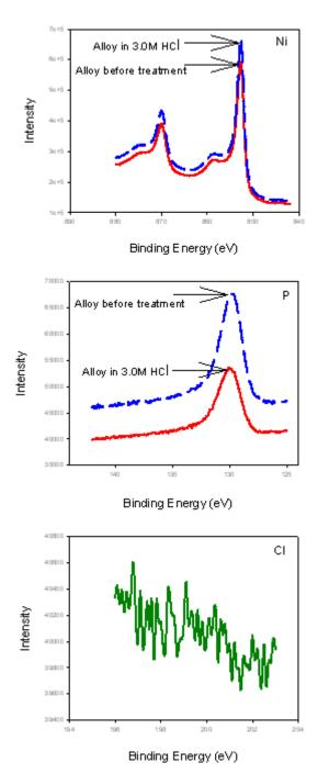
Fig. 2: The photo-electron spectra obtained for Ni<sub>89</sub>P<sub>11</sub> glassy alloy before and after the experiment in 3.0M HCI.
