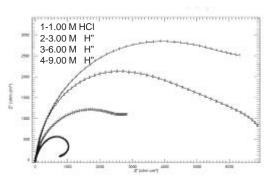
Fig. 3: Impedance plots of Ni<sub>89</sub>P<sub>11</sub> glassy alloy in different concentrations of HCI.
