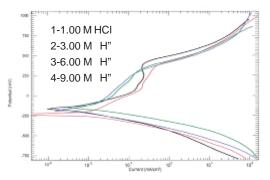
Fig.1: Potentiodynamic polarization curves of  $Ni_{R0}P_{11}$  glassy alloy at concentrations of HCI.
