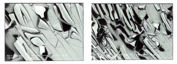
Fig. 4: Scanning electron micrographs of Ni<sub>89</sub>P<sub>11</sub> glassy alloy at different magnifications in 3.0 M HCl solution.
